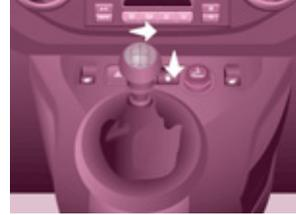
To engage reverse gear, wait until the vehicle is stationary then push the gear lever to the right then down.
