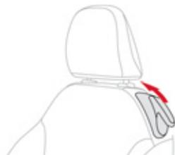
Pull the control upwards to fold the seat back and move the seat forward.
