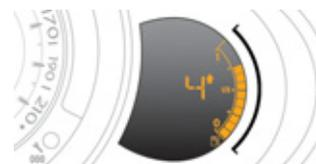
System which reduces fuel consumption by advising the driver to change up on vehicles fitted with a manual gearbox.
